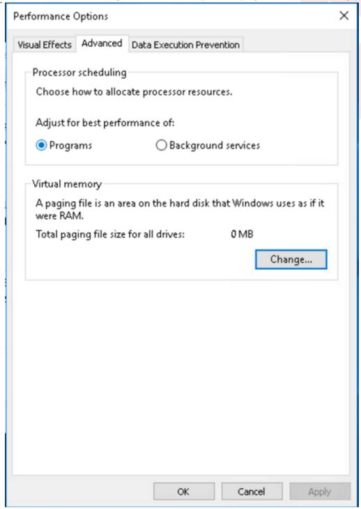
6. From the Virtual Memory panel, uncheck the option to **Automatically manage paging file size for all drives**.
