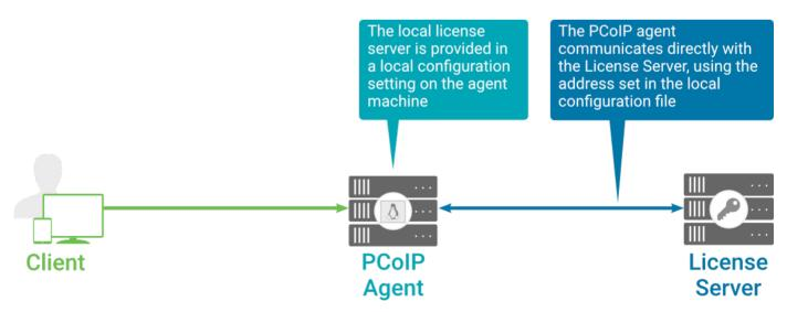
Local license validation using a Standard Agent for Linux and a direct (unbrokered) connection
