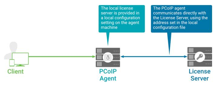
Local license validation using a Standard Agent for Linux and a direct (unbrokered) connection
